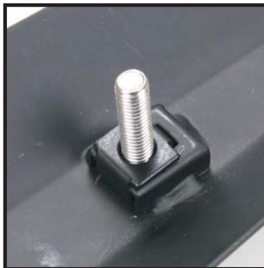
Insert the anti-rotation lock adapter so that it does not allow the bolt to spin freely. The adapter can only insert 1 direction so take note of the tab widths.
