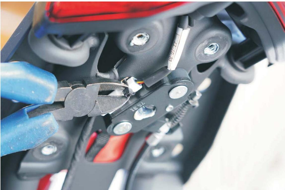
8. Place the Mounting Bracket between the tail light harness and sub frame and mount it using the same 4 factory bolts removed from step 5 above. Due to loose tolerance levels on Ducati's craftsmanship in welding we faced clearance issues with some 1200R models. Perform a clearance test next.
