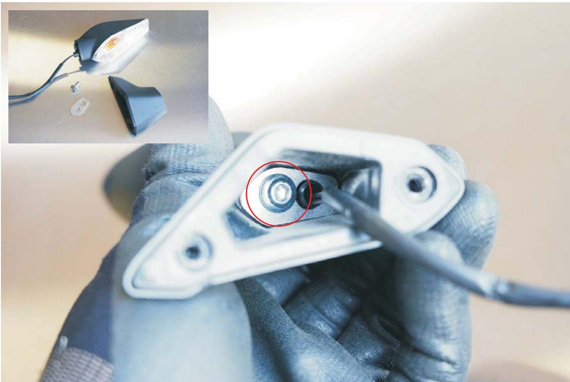
15. Install the turn signals onto the appropriate factory turn signal bracket from this kit using the supplied spacers and secure with bolt removed from step 14 above. Left and right turn signals are different, make sure to install accordingly so the drainage hole on the lens is facing down.
