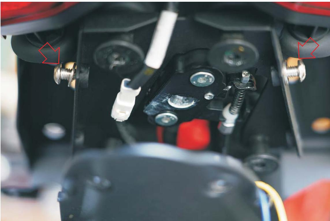
10. Attach the Plate Holder to Plate Support using three (3) M6x12mm bolts, M6 washers and M6 lock nuts making sure to center the holes up. Use 4mm allen and 10mm socket to tighten.
