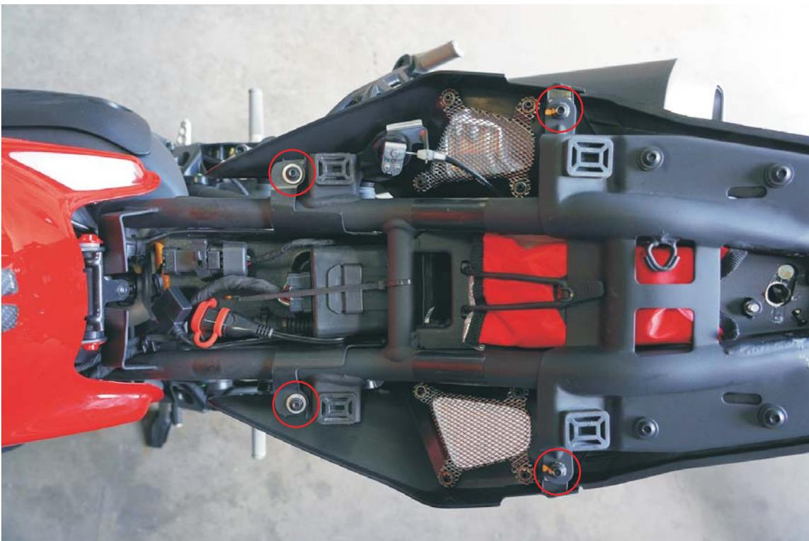
2. Remove under tail continued (4mm allen tool - 2 bolts from the bottom), then carefully drop down the under tail
