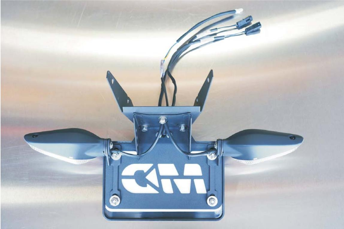
17. Place towel over tire/muffler, then rest fender eliminator assembly on top. Plug in the left/right signals and license plate light. DX to 530.1.022.6B (right) and SX to 530.1.023.6B (left)
