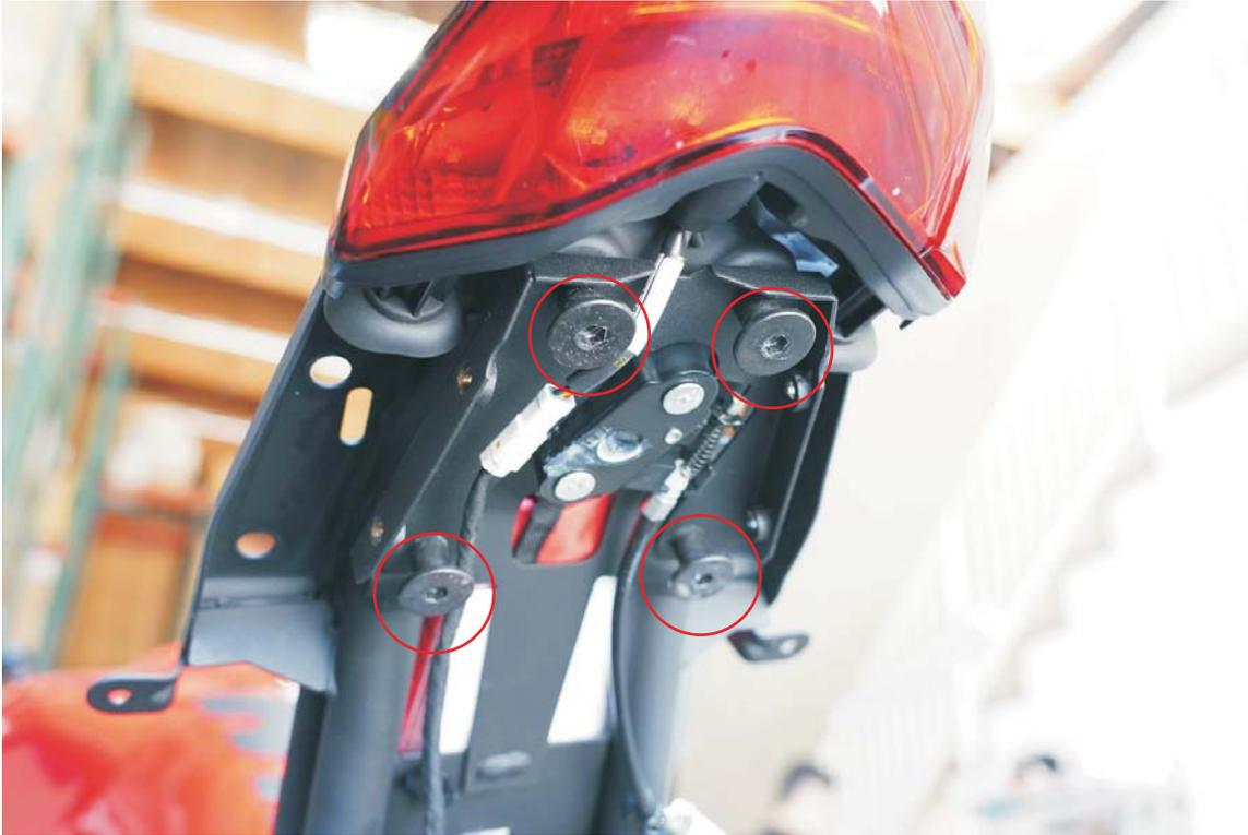
9. \*Clearance test - grab two M6x12mm bolts and try threading into the 2 rearmost holes of the Mounting Bracket. If you are able to screw the bolt without interference then continue to the next step otherwise you will need to install four(4) M6 washers between the Mounting Bracket and sub frame.
