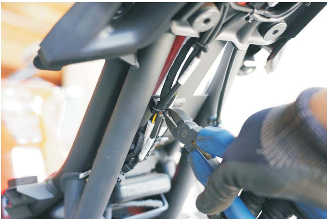
4. Unplug left/right signals and license plate light plugs (2 black signal plugs and 1 white license plate light plug). TIP: Compress the locking tab on connectors to unplug.
