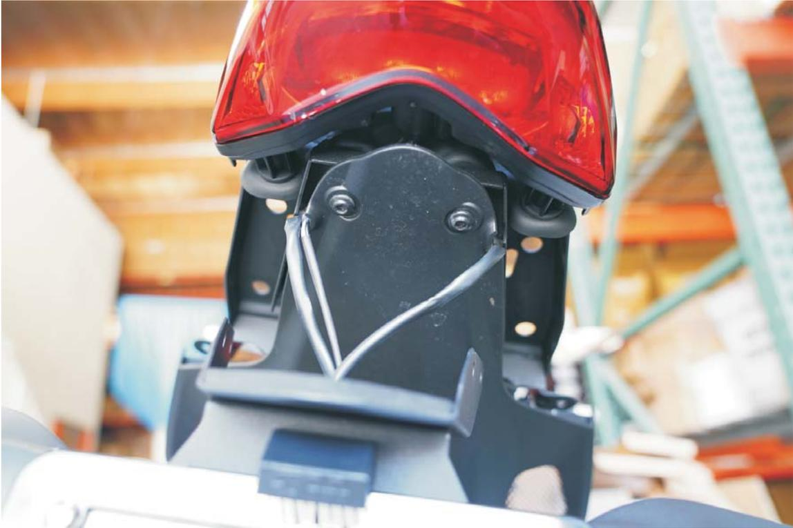
19. Mount the plate holder assembly to the Mounting Bracket using four(4) M6x12mm bolts and M6 washers. Apply a drop of Loctite or thread sealer on these bolts. Before final tightening push up on the fender eliminator assembly to eliminate the gap under the tail light.
