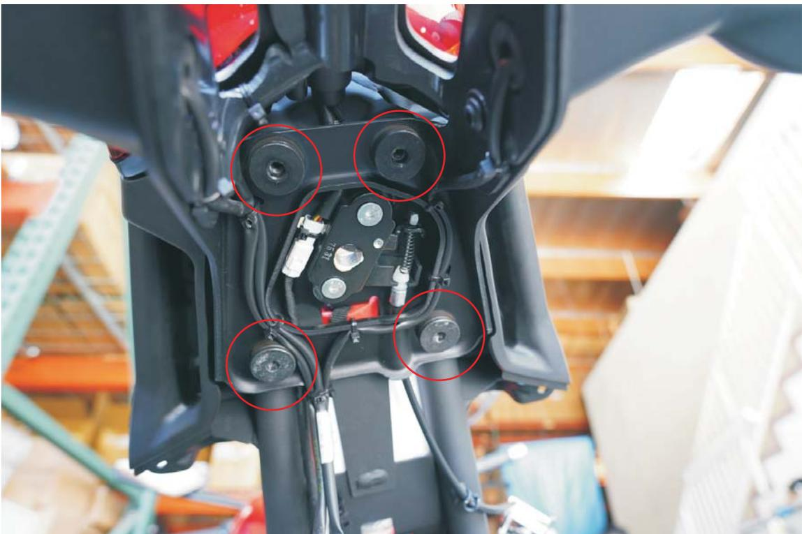
6. Remove grab handles (4mm allen tool - 2 bolts from the top for each side). Note: these have a shouldered spacer under these bolts to assisting aligning the grab handles when reinstalling later
