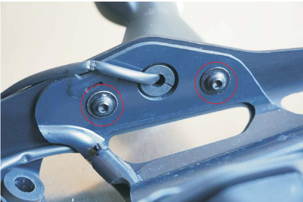
14. Remove the neck of the turn signal (1 bolt from inside) - retain bolt for reinstalling, the special washer is no longer needed. This bolt has Loctite so using a socketed 4mm allen will aid to break it loose. Repeat on other side.
