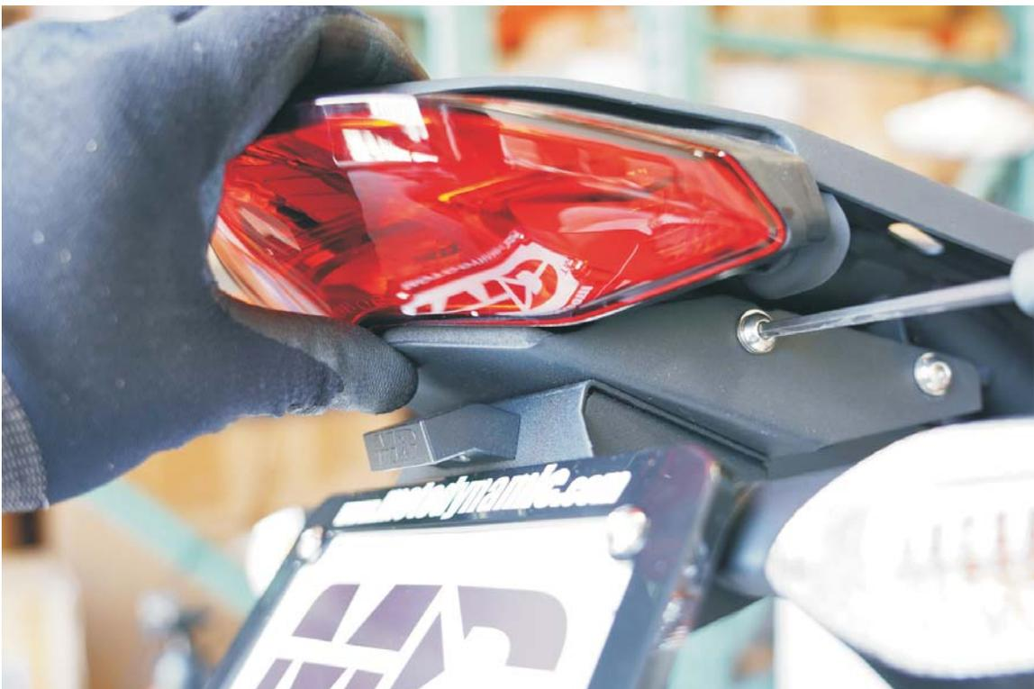
20. Finish re-installing the under tail (4 bolts from up top)
