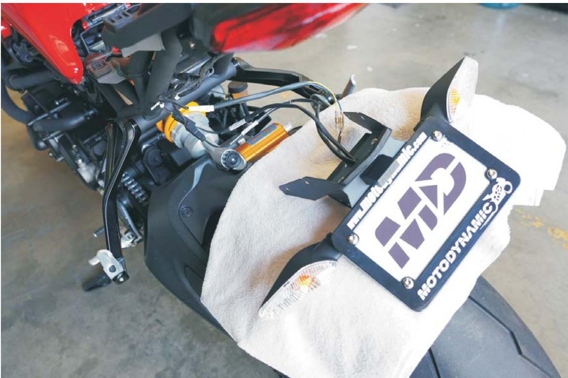
18. Place the under tail back ensuring left/right signal and license plate light wires are divided. Group the license plate light wire with the left signal. Tighten the two(2) rearmost bolts of the under tail. Reach in from the left side forward end of the under tail and pull 3 harnesses to take up the remaining slack while supporting fender eliminator assembly.
