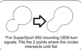
\*For SuperSport 950 mounting OEM turn signals. File the 2 points where the circles intersect until flat
