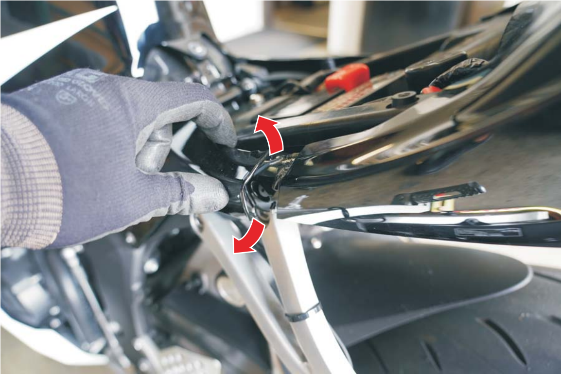
Step 3 continued (flexing upwards on the side fairing helps to clear it from the body)
