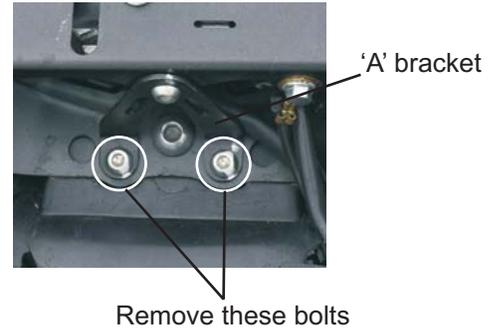
5. Run the wire(s) back up through the under tail and mount the plate holder assembly to the bike using the (2) M6x14 bolts on the rear facing holes and (2) M6x20 bolts to the front facing holes, M6 washers and lock nuts. Note: The front facing holes are threaded and the nut and washer will additionally secure the 'A' bracket from Step 3 above.
