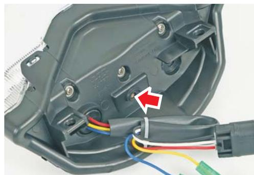
1. Locate the programming button on back housing
