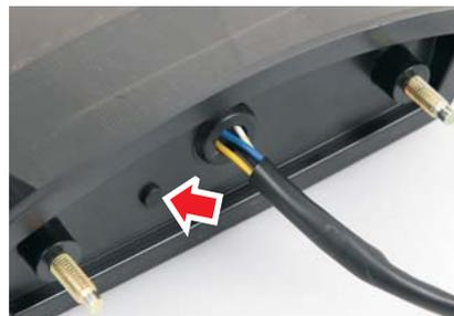
1. Locate the rubber plug on back housing and remove it
