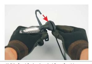
5. Insert/slide front facing bracket from front to rear, until the 2 lower elongated hole aligns from each bracket.
