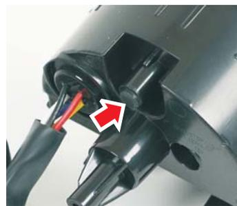
1. Locate the rubber plug on back housing and remove it
