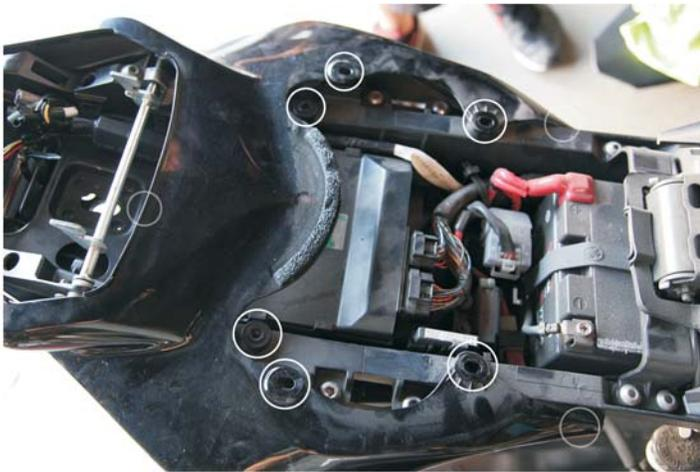
1. Remove factory tail light. Seat removal needed. Upper tail needs to be removed, lower tail needs to be loosened. Remove all plastic rivets and allen bolts that hold down the upper tail. Slide up and back to detach from lower tail.
