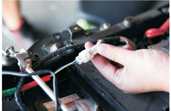
2. Locate factory tail harness and disconnect. Locate left and right signal connectors (black and gray) and disconnect. Unbolt and remove factory signals.
