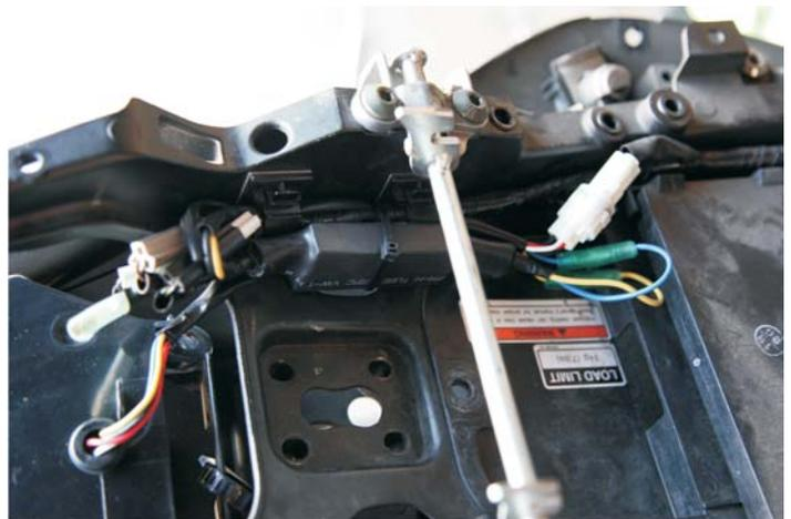
4. Connect main 3-wire harness. Secure subharness with cable ties, etc and reverse procedure for reinstalling the tail lamp. Transfer the foam block (06-07) to new LED tail light and use additional adhesive if necessary. Test all functions before re-assembling upper tail.
